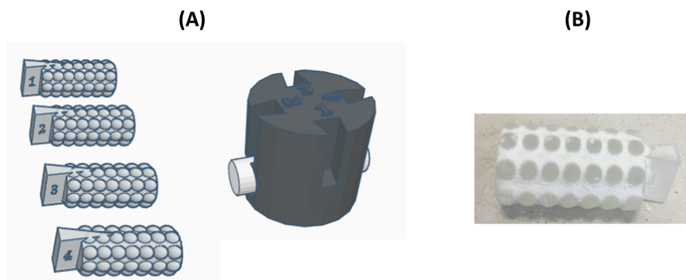
Figure 1. (A) CAD design of the extraction device (paddles and magnet-containing holder) and (B) polymer-coated 3D-printed paddle.
